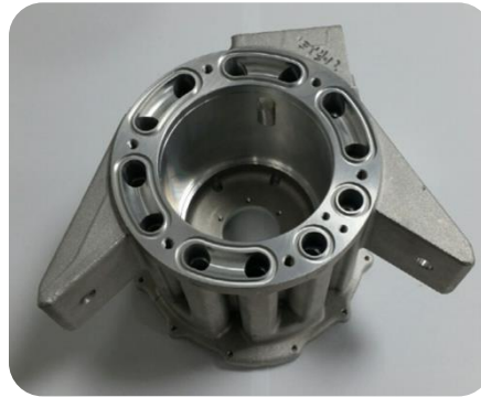
Motor Housing (Finish Machined(f))
